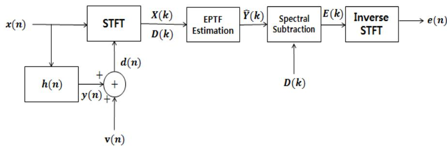
Figure 1. Block diagram of the conventional method
