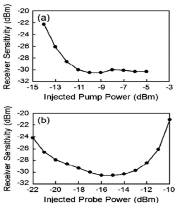
Fig.5. (a) Measured receiver sensitivity as a function of the injected pump power into the RSOA when the probe power is dBm. (b) Measured receiver sensitivity as a function of the injected probe power into the RSOA when the pump power is
