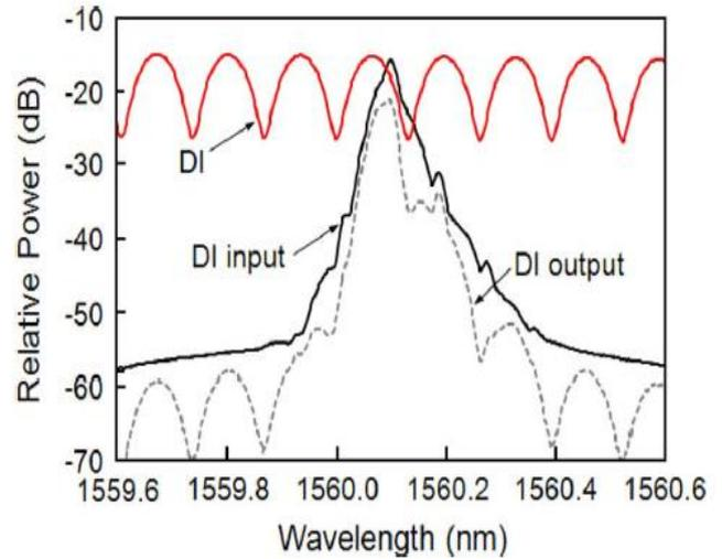
Fig.3. Measured optical spectra at the DI input (solid black) and at the DI output (dashed grey). The transmittance curve of the DI is plotted in red.
