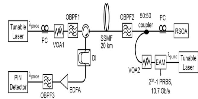
Fig.2 Experimental setup DI: delay interferometer, EAM: electroabsorption modulator, EDFA: Erbium-doped fiber amplifier, OBPF: optical band-pass filter, PC: polarization controller, PRBS: pseudo-random binary sequence, RSOA: reflective semiconductor optical amplifier, SSMF: standard single-mode fiber, and VOA: variable optical attenuator.
