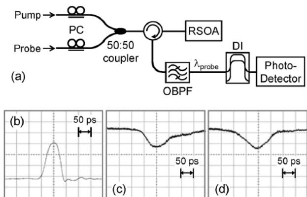
Fig. 4. (a) Experimental setup to measure the gain recovery time of the RSOA. (b) Waveform of the 60-ps pump signal. (c) Waveform of the probe signal before the DI. (d) Waveform of the probe signal after the DI.
