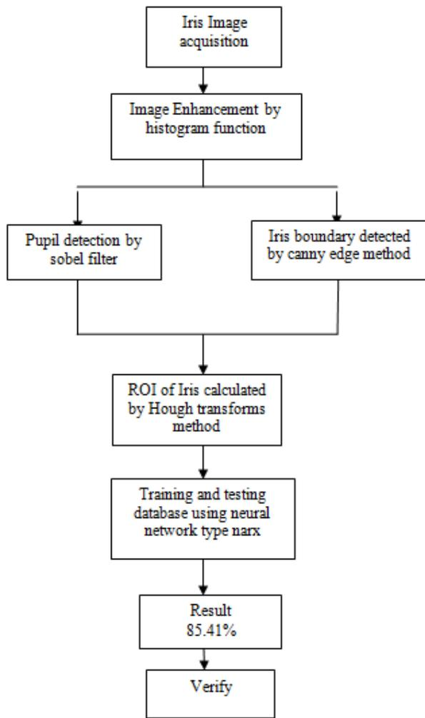
Figure 1. Flow chart of Iris recognition system
