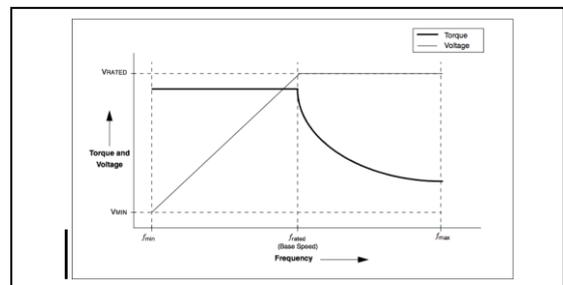
Figure 3 Torque speed characteristics of induction motor
