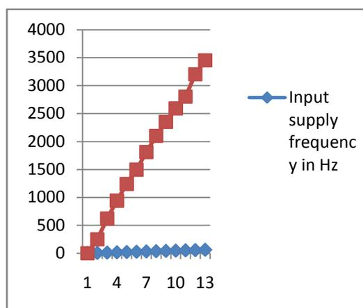
Figure 6 Frequency input vs. speed output
