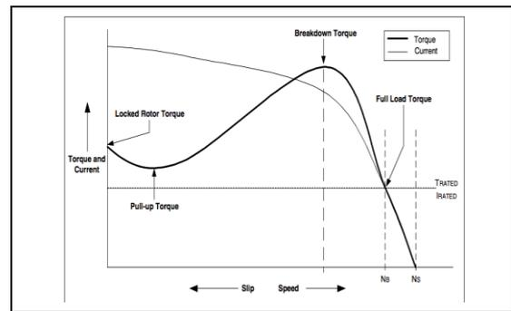
Figure 2 Torque speed characteristics of induction motor
