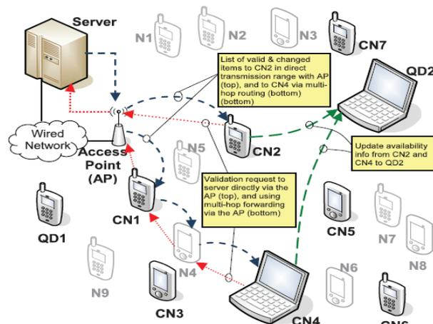
Figure1. Design Structure
