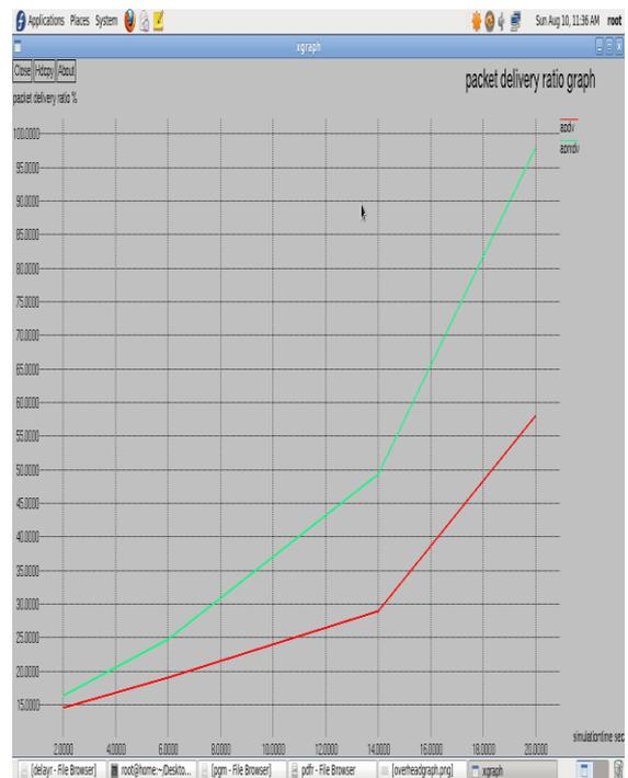
Packet delivery ratio varying with simulation time
