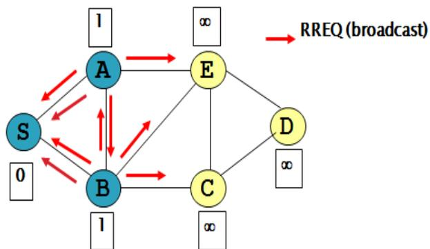
Figure4. Route Request control packet in AODMV
