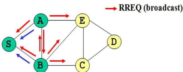
Figure2. Route Request control packet in AODV
