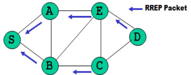
Figure3. Route Reply control packet in AODV
