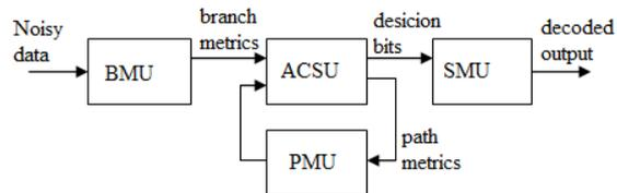
Fig.5. Block diagram of viterbi decoder
