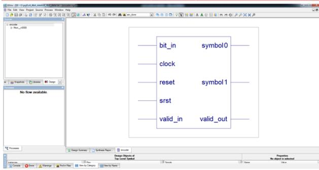
Fig.6. RTL Schematic of convolutional encoder
