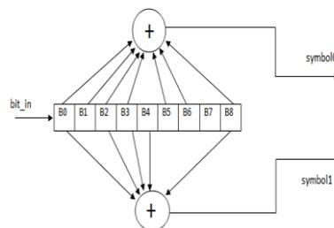
Fig.3. Proposed convolutional encoder
