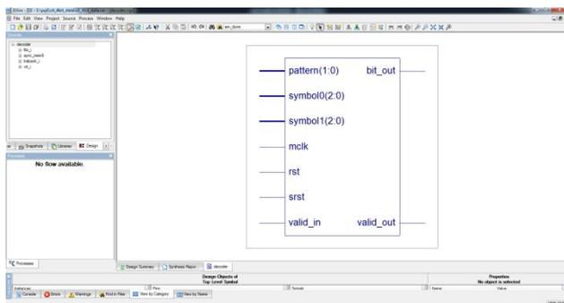
Fig.8. RTL Schematic of viterbi decoder
