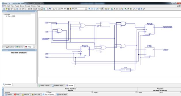
Fig.7. Internal structure of convolutional encoder
