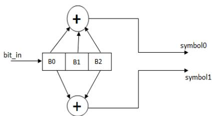
Fig.2. Basic Convolutional Encoder
