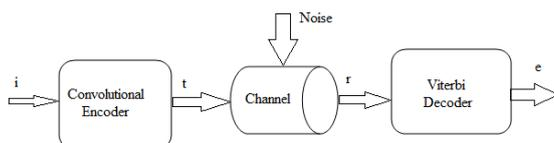
Fig.1. Basic communication system with encoder and decoder
