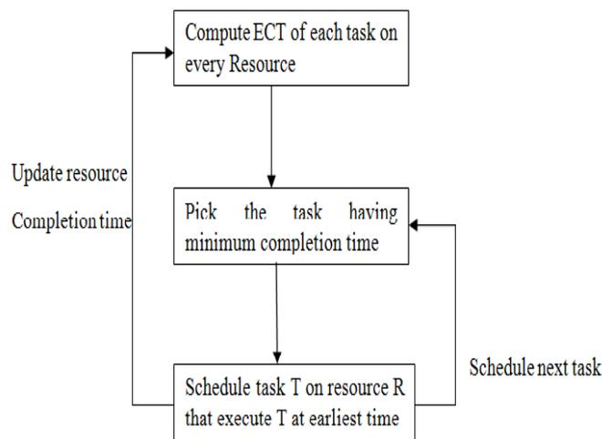
Figure. 1 Min-Min Scheduling Algorithm
