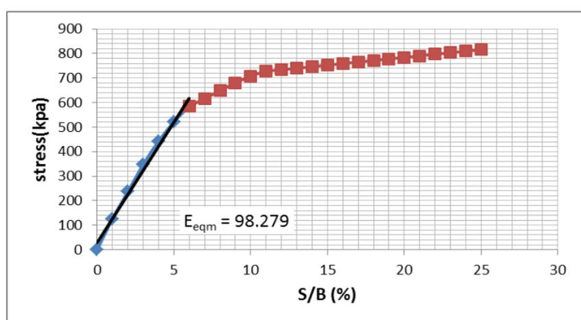
Fig. 5: method of determining  $E_{eqm}$
