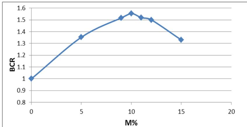
Fig. 5: Effect of tire chips with sizes in the range of 4 to 9 mm on BCR
