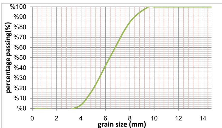
Fig.3. Grain size distribution curve for tire chips
