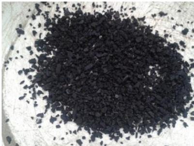
Fig.2: View of tire chips with sizes in the range of 4 to 9 mm
