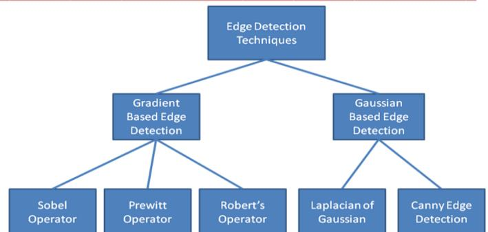
Figure 1 Classification of Edge Detection Techniques
