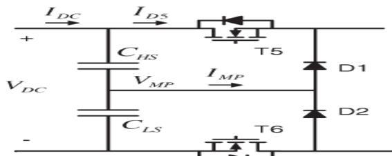
Fig.8. DC capacitor circuit employed for the analytical analysis of the Voltage Balancing.
