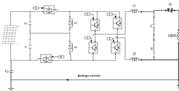
Fig.5.Schematic diagram of PV-grid connected H6 topology
