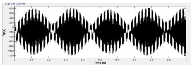
Fig.6 (a).H5 topology parasitic voltage
