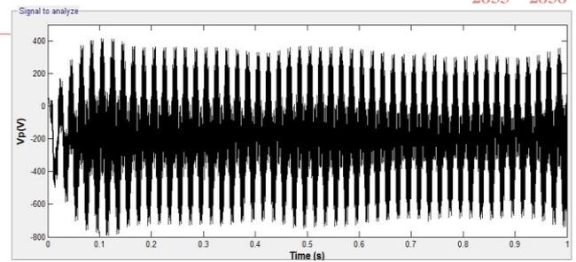
Fig.6 (c).H6 topology parasitic voltage
