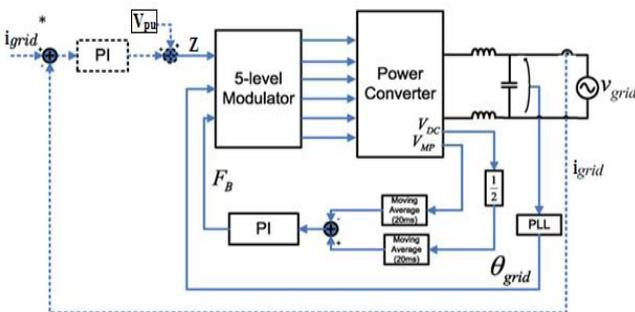
Fig.9. Block scheme of the balancing control of the midpoint voltage
