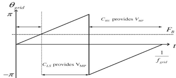
Fig.10. MVC working in case of a positive  $FB$
