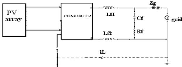
Fig.1. Path of the common mode current in transformer-less system
