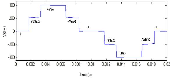
Fig.3. generalized single phase multi level inverter output voltage
