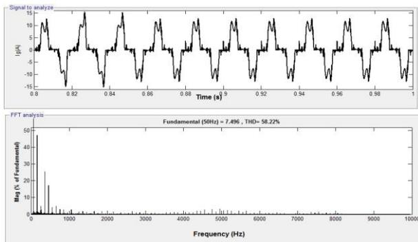
Fig.11(c).grid injected current
