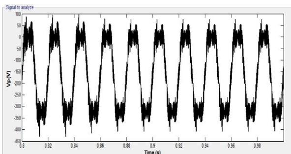
Fig.11(e).parasitic capacitor voltage
