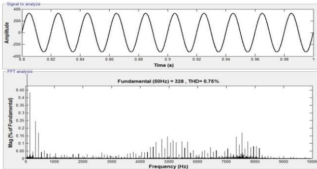
Fig.11(b): the grid injected voltage with FFT analysis
