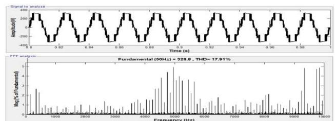
Fig11a: The H6 converter output voltage with FFT analysis
