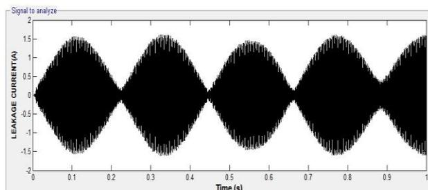
Fig.6 (b).H5 topology leakage current
