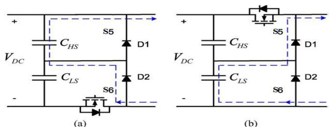
Fig.7. S5 and S6 configurations providing the same voltage  $V_{MP}$  to the full bridge rails. In (a), the HS capacitor is discharging, and in (b), the LS capacitor is discharging
