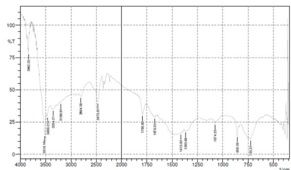
Fig. 2 FTIR spectra for CdO nps
