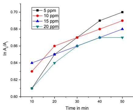
Fig. 5c Curve fit data for the first order degradation kinetics of methyl red
