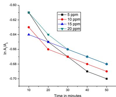
Fig. 5b Degradation of methyl red as a function of  $\ln(A_t/A_o)$  versus time of exposure to UV light
