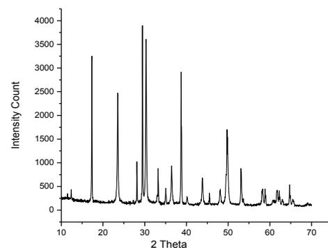
Fig. 1 XRD pattern for CdO nanoparticle
