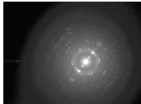
Fig. 4c. SAED pattern of CdO nanoparticle
